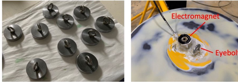
Fig. 8. Photos of steel disks used to attach to the electromagnet and installation of electromagnet and eyebolt
