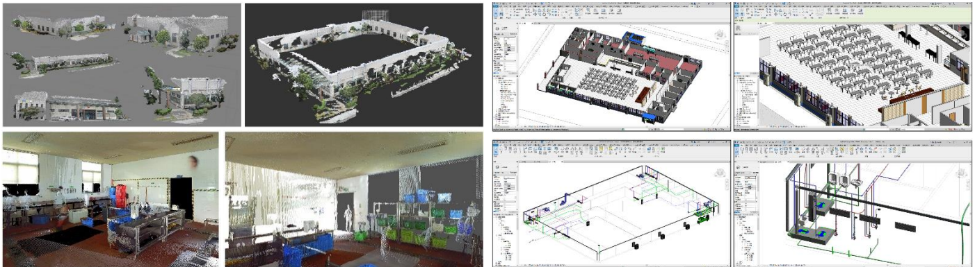
Figure 5. Staff restaurant external and internal Recap scanning results and Revit model
