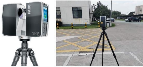
Figure 3. Use FARO Focus3D X 130 Laser Scanner to create point clouds
