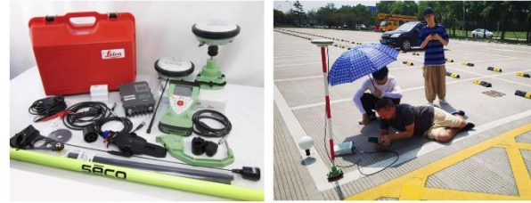
Figure 4. Use Leica GS14 GNSS RTK to collect on-site data
