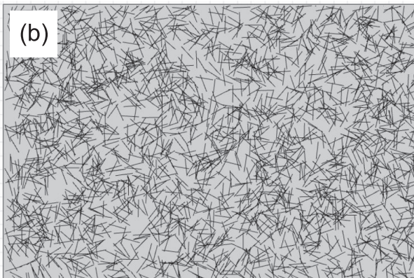
Fig. 7. Schematic diagram of the randomly distributed fiber-reinforced bentonite. (a) single fiber, (b) randomly distributed fiber model.
