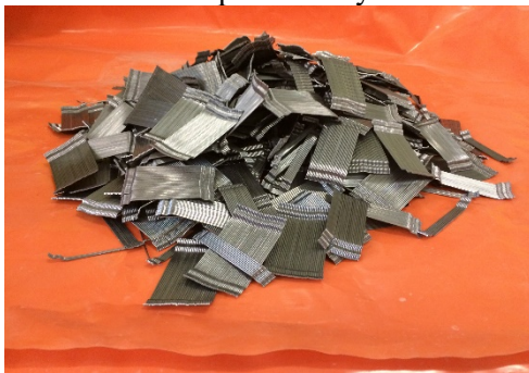
188 189 Fig. 1. (a) 4D steel fiber (b) Single part of fiber with 60 mm length 190 191
