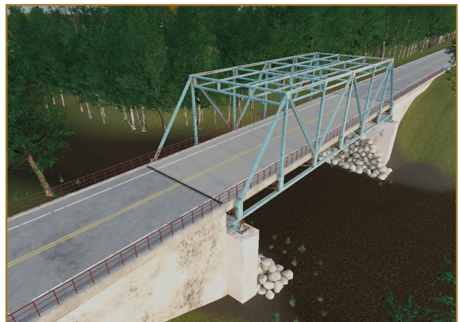
Top view of the final version of the steel bridge modeled within the virtual environment.
