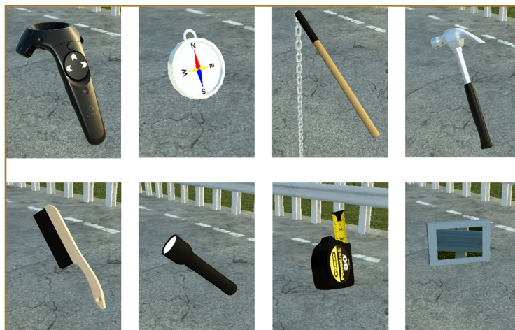
VR headset controller and inspection tools modeled. From top to bottom and left to right: controller, compass, chain drag, hammer, scratch brush, flashlight, tape measure, and zoom window
