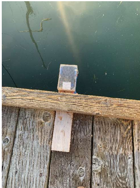
Figure 20: Cantilever Instrument Mount at the Coast Guard North T-Pier
