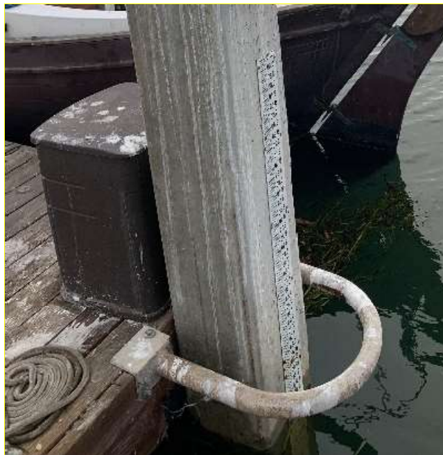
Figure 24: Tide Staff at the Coast Guard North T-Pier (Before Cleaning)
