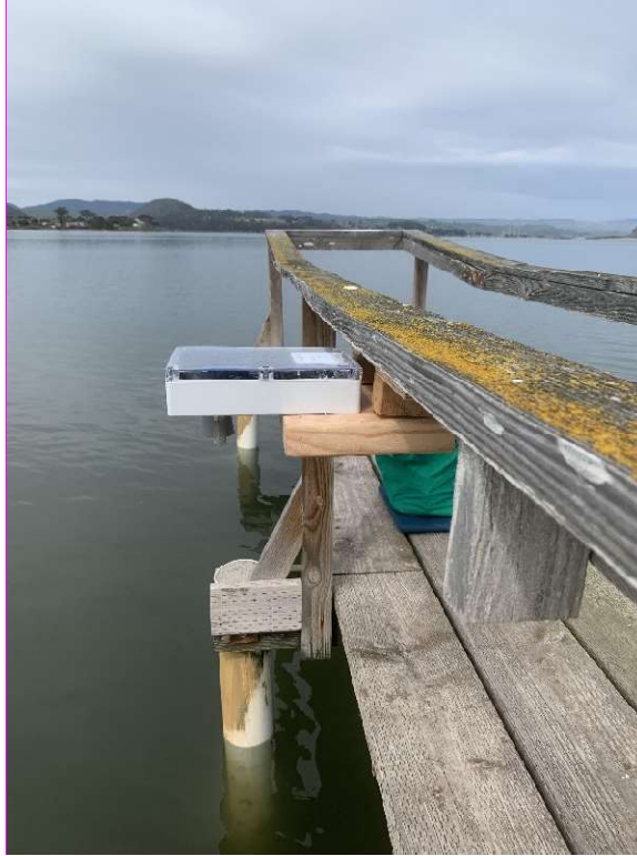
Figure 22: Cantilever Instrument Mount at the Private Pier in Los Osos
