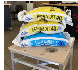
118.8 Pound Load on Metal Frame and Top Shell Panel
