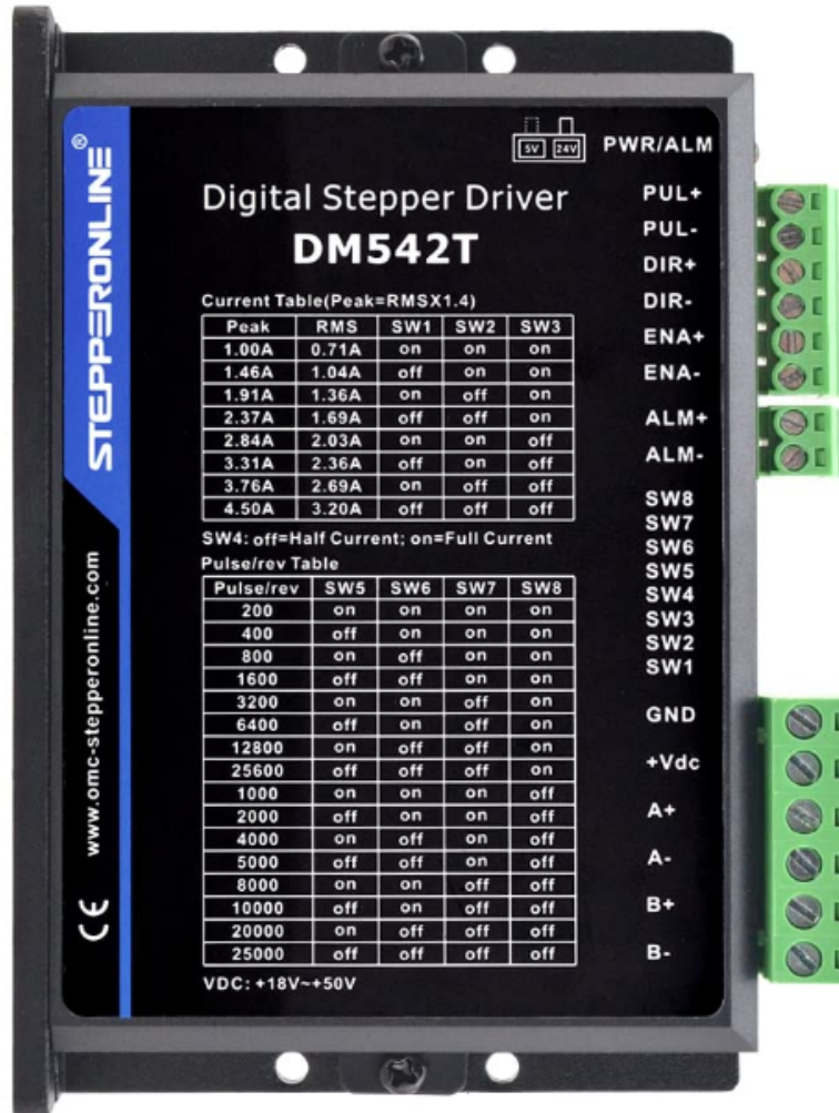
Figure 4.7: Fully digital stepper driver, manufacturer part number DM542T-23HS45, developed with advance DSP control algorithm offering automatic idle-current reduction, over-voltage and over-current protections, soft-start with no jump in step when powered on, and micro stepping capability up 25,000 steps per revolution [7]
