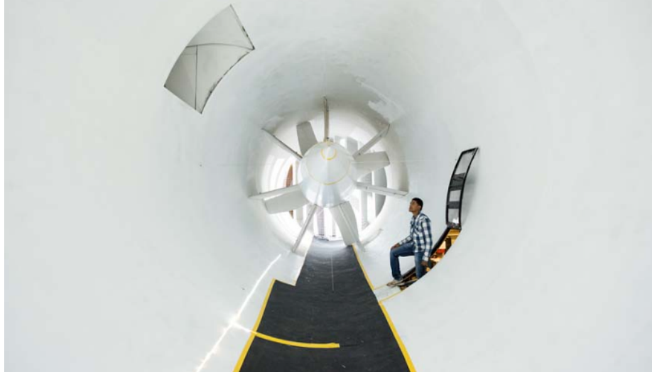
Figure 3.8: Former Ph.D. researcher Nandeesh Hiremath entering the main diffuser section of John Harper Wind Tunnel Memorial near the tunnel's four blade driven fan powered through a World War II Curtis bomber propeller hub [34]
