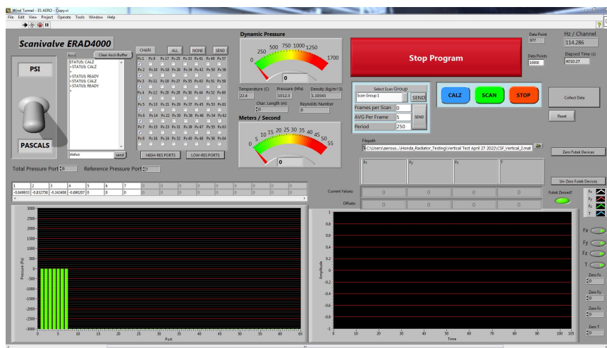
Figure 4.14: LabVIEW terminal interface with controls of zeroing load cell, setting sampling rate, and saving data points to mat file
