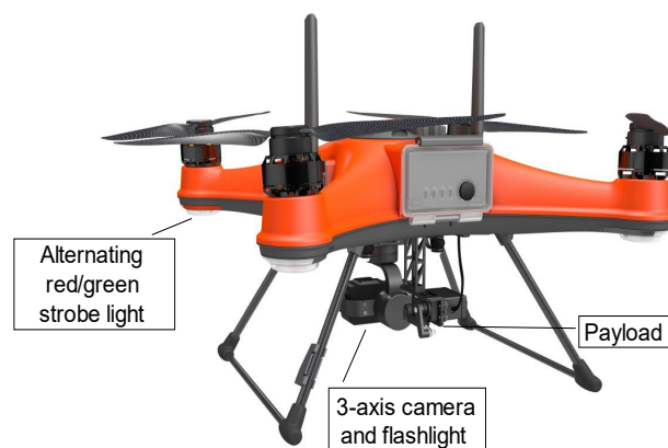
Figure 1. SwellPro SplashDrone 4 with diagram of pertinent features.
