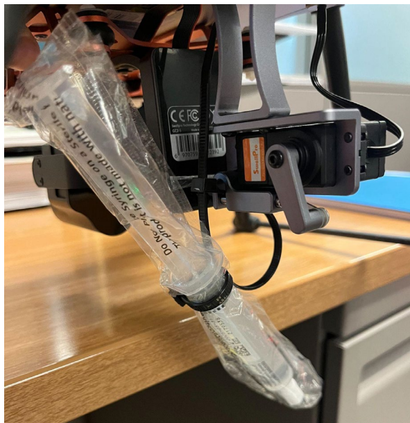
Figure 3. Example of simulated antidote (10 milliliter normal saline syringe) attached to UAV payload by plastic cable-tie.
