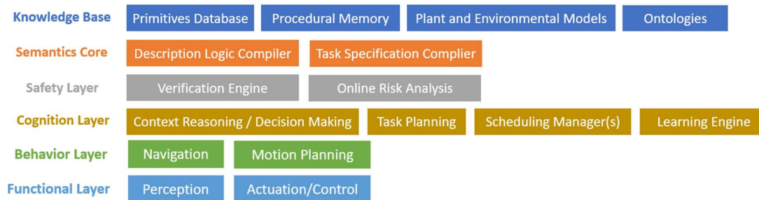
Figure 1(c). Autonomy stack from (Barad, Martinez Luna, Dentler, & Olivares Mendez, 2021)
