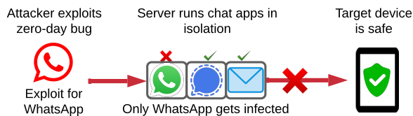
Figure 2. Envisioned Zero-Click Secure Framework: Users access remote, isolated apps via screen sharing, limiting zero-click exploit to the targeted app.
