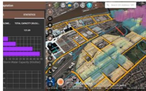
Figure 6. Real-time Water-sensitive Urban Design Decision Support Tool developed on a spatially enabled Digital Twin. Source: Rahmani, 2023
