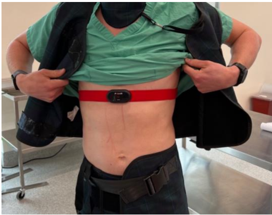
Figure 1: Study participant wearing a Polar Team Pro strap and transmitter. The black centerpiece is known as a “puck” which processes, stores, and transmits all the data.
