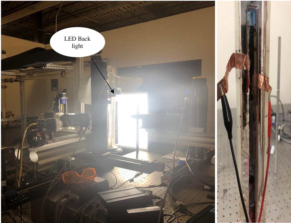
Figure 3.4: The PIV facility with LED back light on (left) and a back-view of the test section (right).
