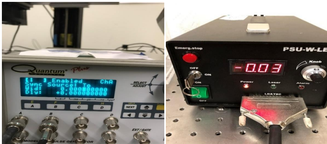
Figure 3.5: The external pulse generator (left) and the continuous laser ( \lambda= 532 nm, 10W).
