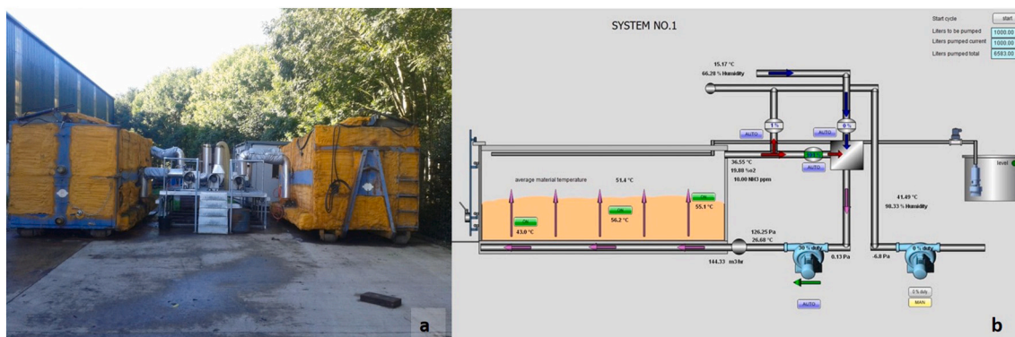
Fig. 1. Pilot scale containers incubators with temperature, aeration and odour control ventilation in the centre (a) and the control system (b) used.
