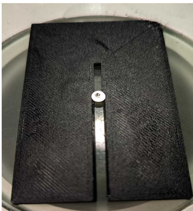
Figure 5: 3D printed gasket holder with a preindented gasket.
