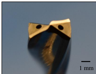
Figure 36. Drill (8 mm diameter) with dual coolant holes
