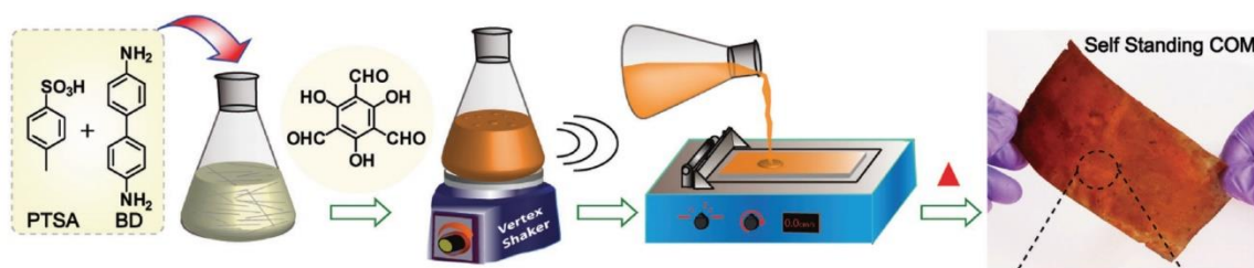
Figure 8. Schematic representation of the COMs (M-TpBD) fabrication. Reproduced from Kandambeth, S.; Banerjee, R. et al., Adv. Mater. 2017, 29, 1603945. 3 With permission from John Wiley and Sons.
