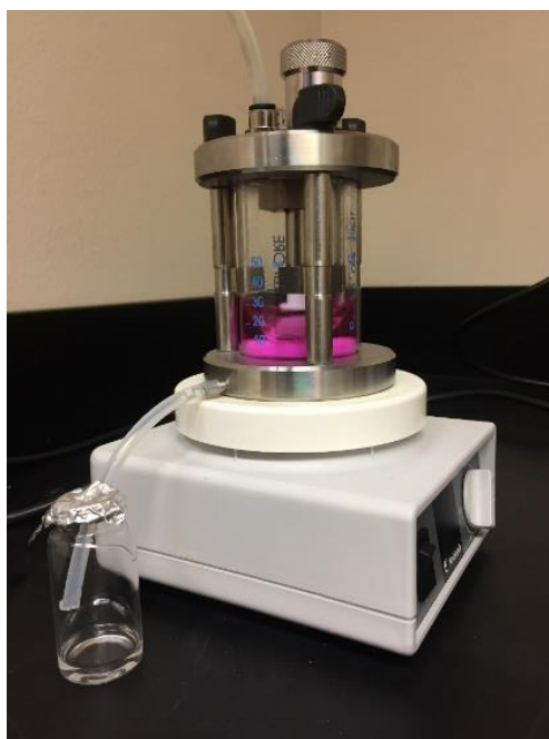
Figure 48. Photographic image of a p -PPN membrane performing OSN in a solvent resistant
