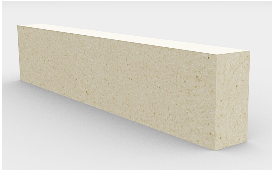
Figure 1 Level Zero of light-weighting with a solid rectangular cross-section.
