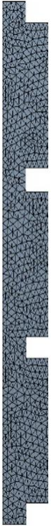
Figure 19. The CFD model of the vinyl siding system. ( l : 2.8 inch, \lambda : 3.3 inch, s : 0.62 inch, and d : 0.62 inch referring to Figure 18).
