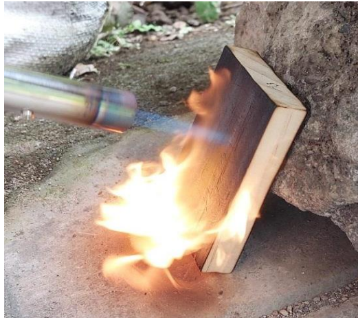
Gambar 1. Pembakaran permukaan kayu sampai hitam merata ( Burning the surface of wood until uniformly black )
