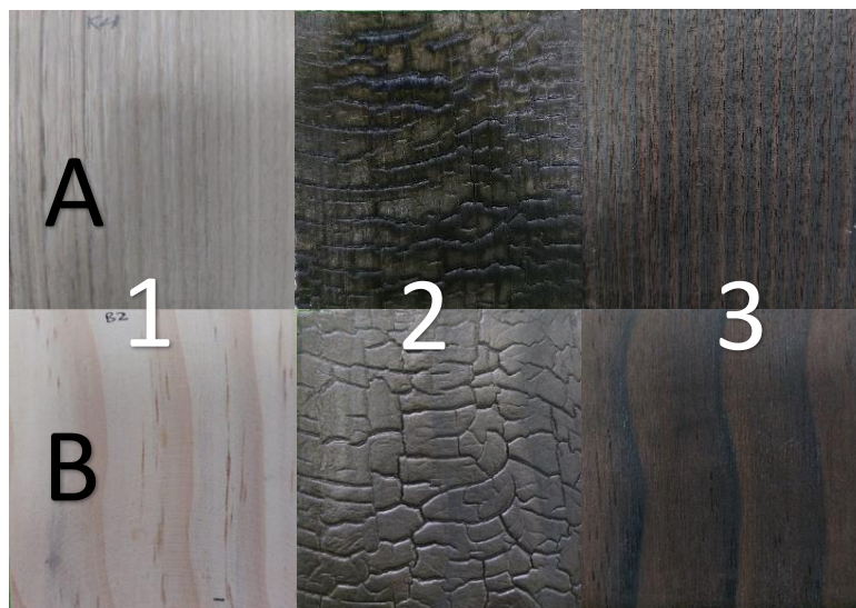
Gambar 3. Proses perubahan tekstur dan warna permukaan kayu sungkai (A) dan pinus (B), sebelum pembakaran (1), setelah pembakaran (2), dan setelah proses pembersihan sisa arang (3) ( The process of texture and color transformation on sungkai (A) and pine (B) wood surfaces, before burning (1), after burning (2), and following the residue charcoal cleaning process (3) )
