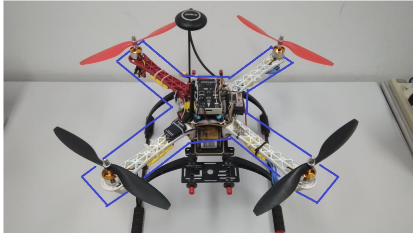
Figure A.2 – Frame of a Quadcopter UAV (highlighted in blue). Source: Author.
