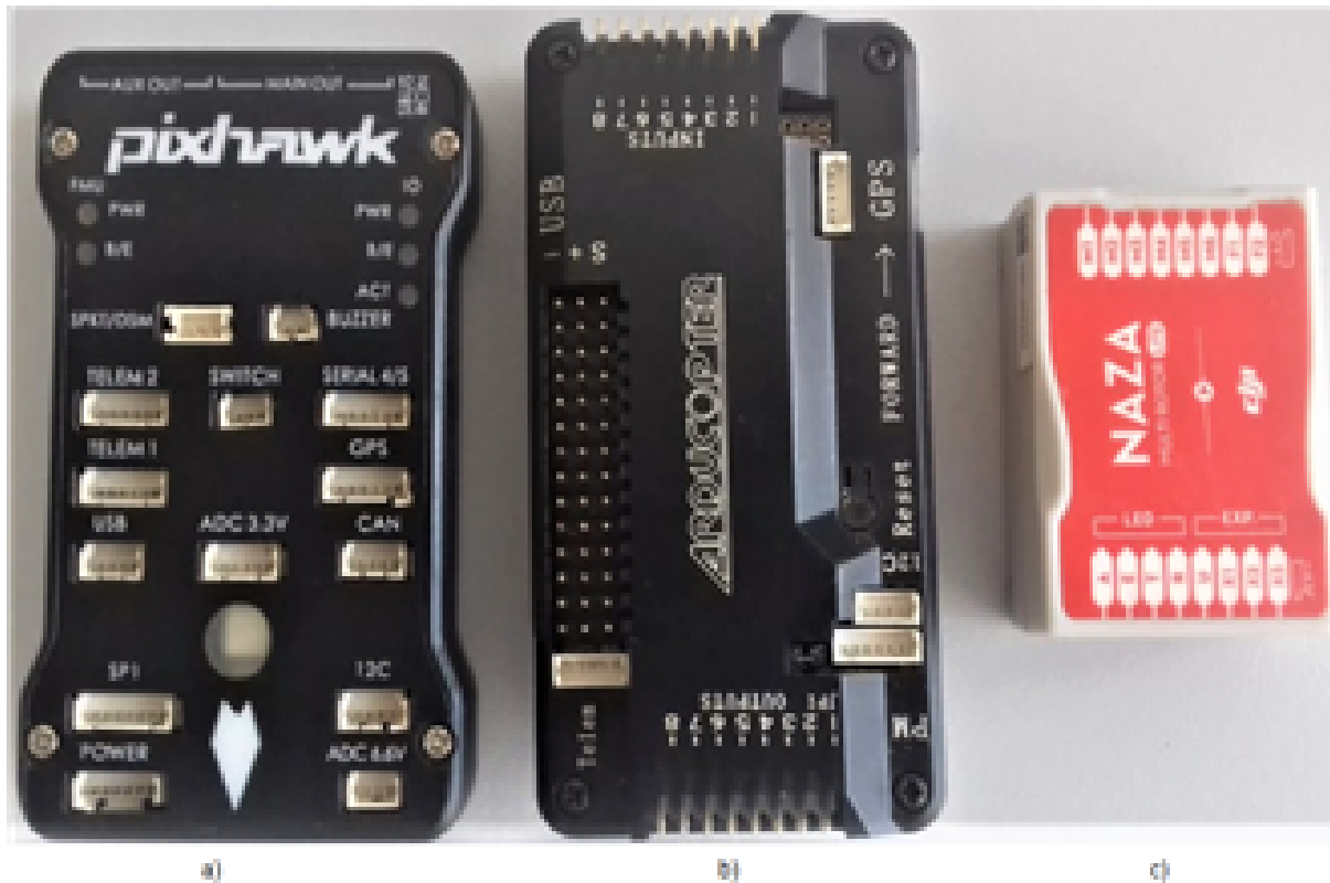
Figure 3.3 – Low cost Autopilots. (a) Pixhawk, (b) Arducopter, and (c) DJI Naza. Source: Author
