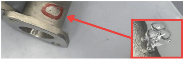
Figure 5 Example of a casting leak (part 9006031) [35]
