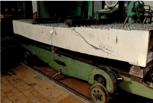
Figure 7a. Typical view of destruction of models tested for bending
