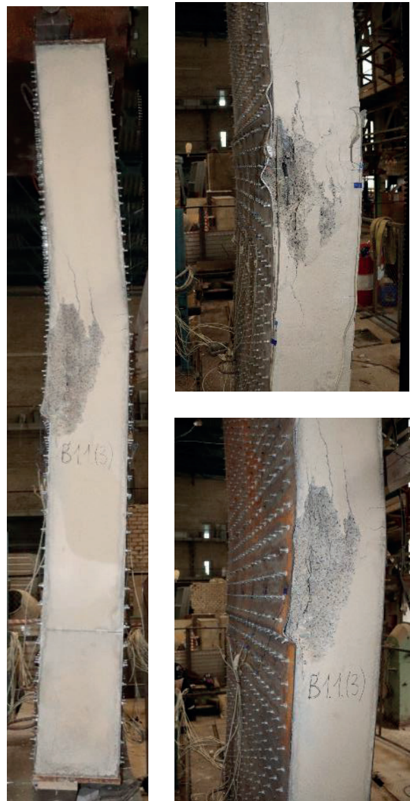
Figure 6. Typical view of destruction of models tested for eccentric compression
