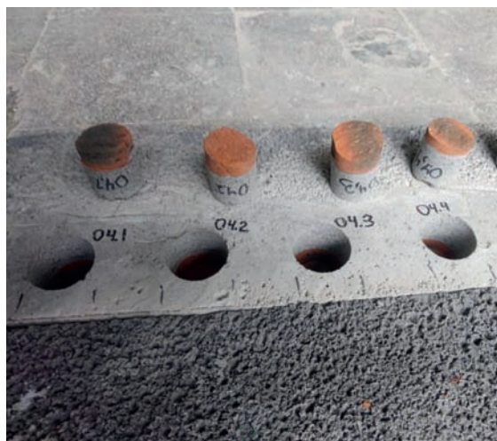
Figure 9. Testing adhesion between shotcrete and brickwork The results can be presented as a diagram (figure 10).
