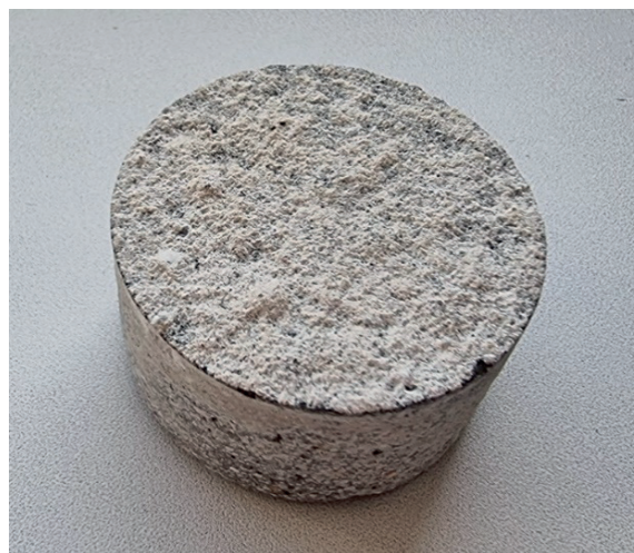
Figure 9. Testing adhesion between shotcrete and brickwork The results can be presented as a diagram (figure 10).
