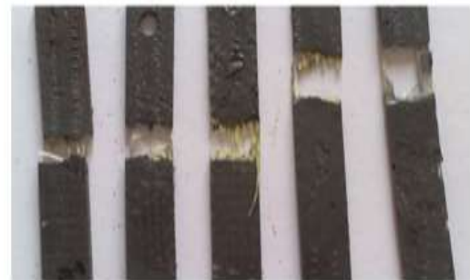
Figure (10) Shows the fracture regions for (EAKG, EAKPVC and EAGPVC) samples
