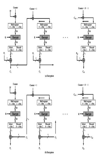
Figure 3: s-bit Counter Cipher Feedback (CCFB) Mode
