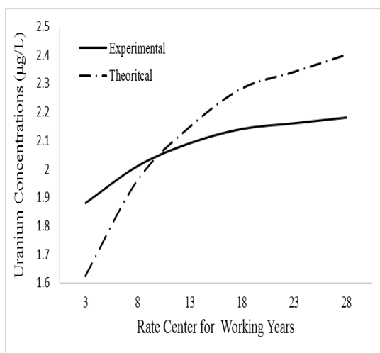
Fig. 3 Comparison between the values, determined by the proposed mathematical model, of uranium concentrations in the urine samples for the X-ray unit workers, and the experimental values of Abdullah [18].
