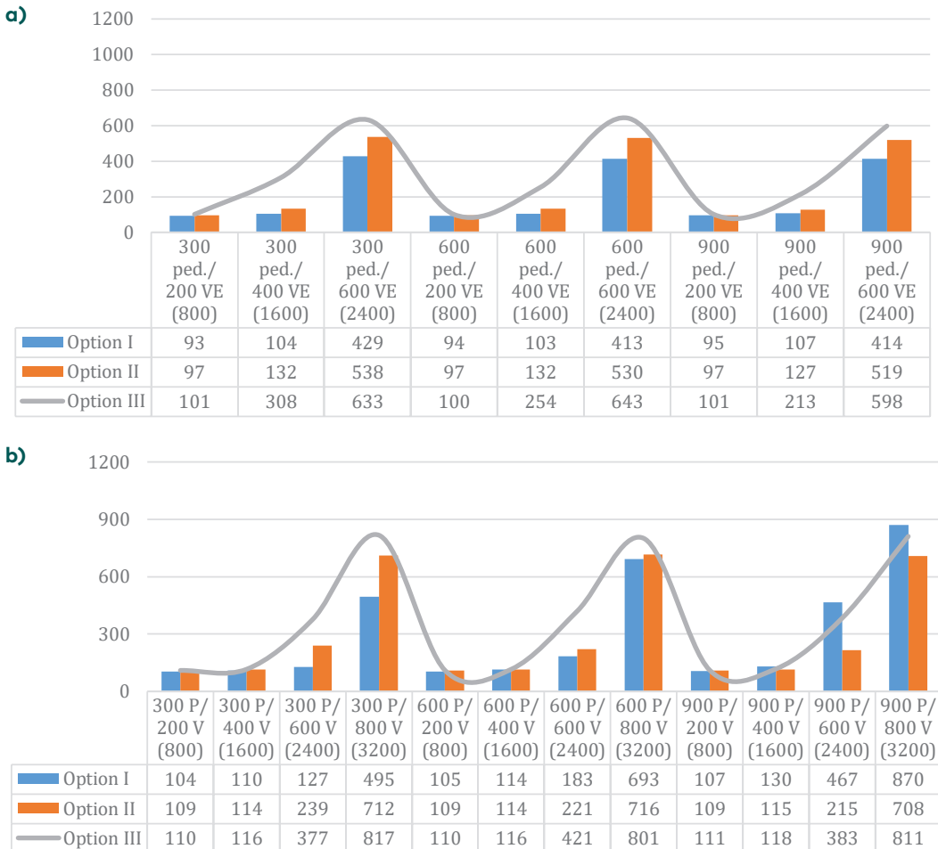
Figure 9. (a, b) Dependence of the travel time, s, of 1V on the geometric parameters of the intersection and the intersection control option for selected combinations of traffic volumes
