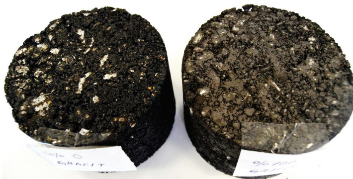
Figure 4. Asphalt specimens with 0% (left) and 100% (right) graphite powder replacement ratios of the filler
