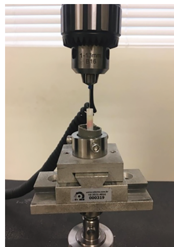
Fig. 1: Evaluation of solvent efficacy through the penetration force using an Instron UTM
