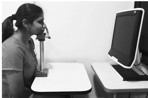
Figure 1. Eye movement perimetry (EMP) setup comprising a thin film transistor (TFT) display with an inbuilt Tobii T120 eye-tracking device. The chinrest was placed at a testing distance of 60 cm. (Participant shown is a volunteer from whom an additional informed consent was obtained for publishing this photograph).
