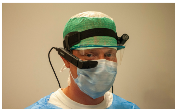
FIGURE 1. An example of a combat medic wearing the Vuzix M400 head-mounted display.
