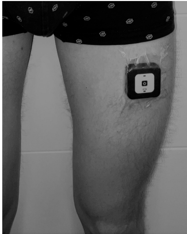
Figure 1. Positioning of 9DoFML device on upper thigh using medical skin tape.
