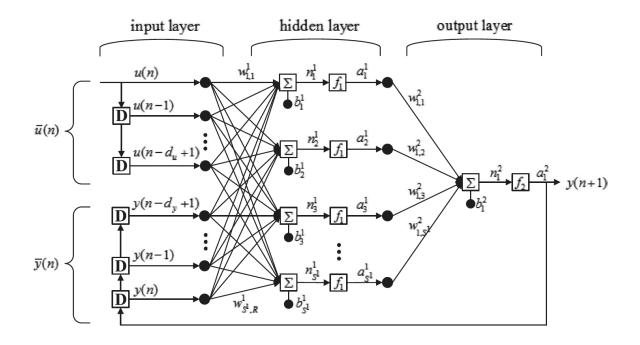
Fig. 3. illustrates the configuration of a NARX [54]
