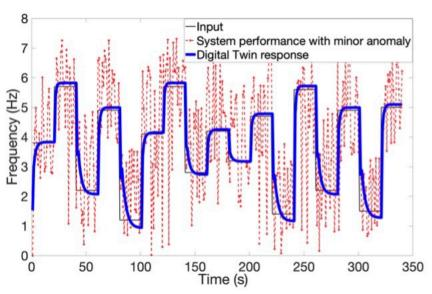
Fig. 16. ICS operation with minor anomaly instances
