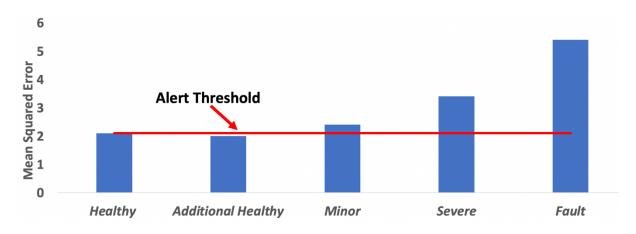
Fig. 20. DT Anomaly Detection, Quantification, and False Positive Mitigation
