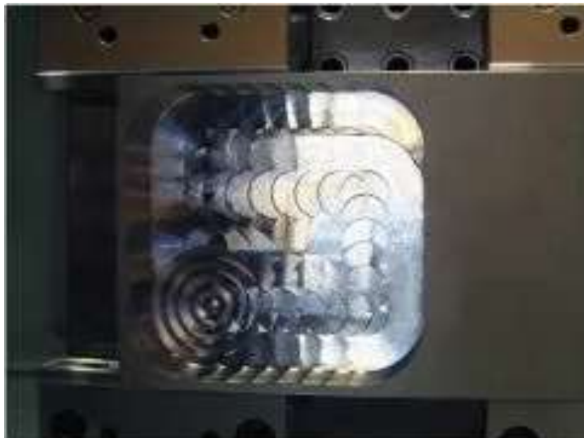
Fig 4.12 Machining a pocket using plunge milling.
