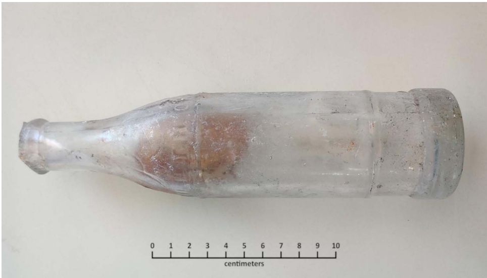
Figure 3. A machine-made soda bottle with “T.H.” embossed on the bottle’s shoulder, dating this bottle to the territorial era in Hawai‘i’s history.
