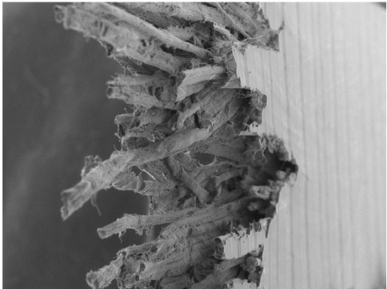
Figure 4.8: The cross sectional optical images (left column) and the fractured area imaged in scanning electron micrographs (right column) of 6 mm curaua aligned discontinuous natural fibre composites.
