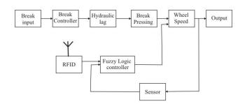
Fig 1.2: Block diagram of a vehicle speed controller with RFID and Fuzzy controller.
