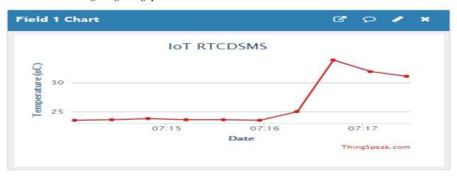
Figure 15: Remote monitoring using ThingSpeak(Temperature parameter)
