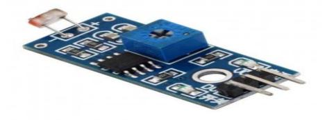
Figure 9: Light Dependent Resistor (LDR) sensors
