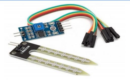
Figure 7: Soil Moisture Sensor
