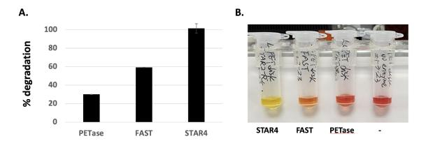
**Engineered PETase enzyme shows improved degradation of PET substrates**. A. Enzymatic degradation of PET powder (3 days) by <u>PETase</u>, FAST and STAR4 enzymes (N=2 ± SD). B. Enzymatic degradation of PET coupon (24 hours) by indicated enzymes in the presence of phenol red pH indicator. Terephthalic acid liberated from enzymatic hydrolysis of PET causes <u>colour</u> change from red to yellow.
