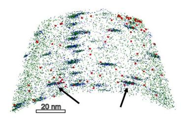
Figure 1 The cryo-APT observation of the titanium carbide in steel with deuterium charging. (red: deuterium, green: titanium, grey: carbon, blue: iron)
