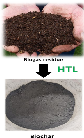
Figure 1 – Production of biochar from biogas residue
