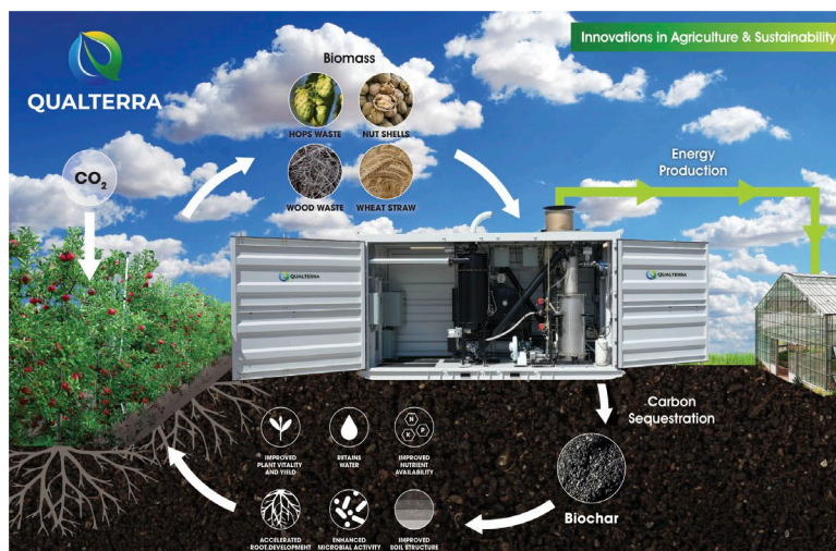
Figure 1– Qualterra's biomass processing technology combines gasification and energy generating processes with modern, automated control systems to convert biomass into renewable energy and biochar. The Biomass Processing Unit (BPU) is housed in a shipping container and is portable and scalable to accommodate a variety of biomass types and site requirements. The BPU is portable and scalable to meet the needs of the end user.
