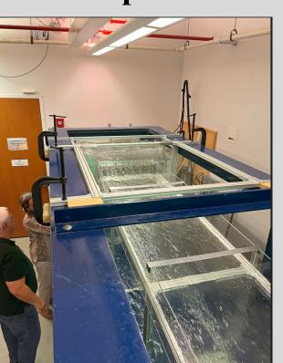
**Figure No.2 & 3: COAS** Wave-lab Water Tank with the Flume, shear sensors and high speed camara ser up.
