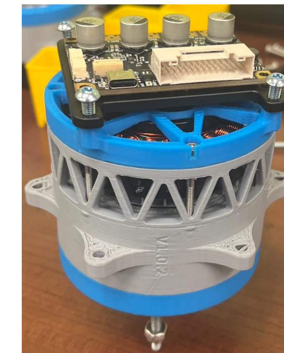
Figure 7: Printed Cycloidal Gearbox
