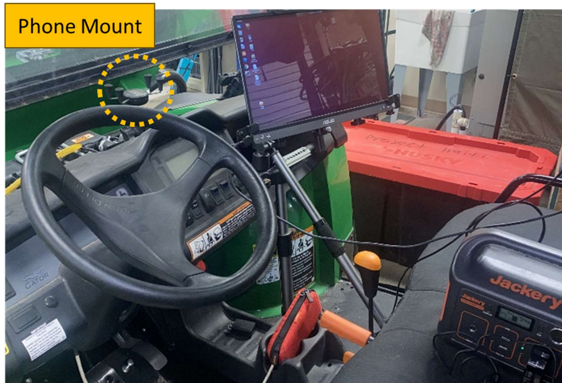
Figure 2.2: Mounting position for phone used as IMU.
