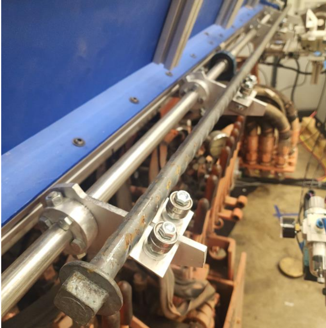
Figure 3.2: A roof bolt waiting for grasping by the robot during the laboratory testing.
