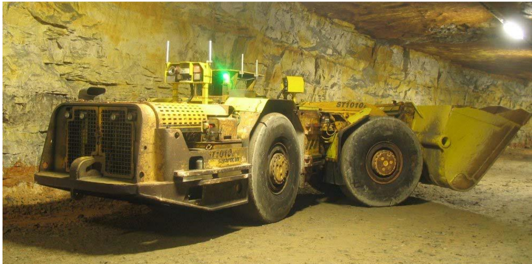
Figure 2.5: LHD vehicle incorporated with sensors and control for autonomous navigation (Larsson, et al., 2008b).
