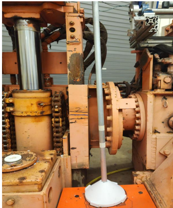
Figure 6.4: Simulated pumpable resin for the automated roof bolting machine.
