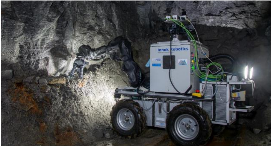
Figure 2.2: An articulated three-finger gripper “Julius” designed to operate like human hands (Grehl, et al., 2017)
