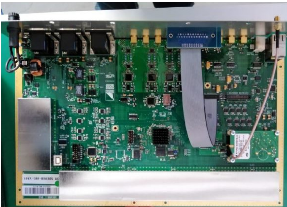
Figure 7. Assembled UUB, equipped with front panel, GPS receiver, cables and shielding covers.
