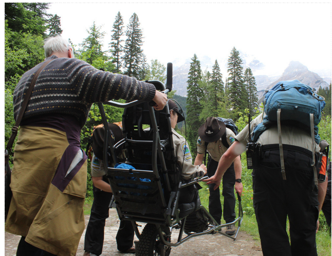
TrailRider is an adaptive single tyre 'wheelchair' designed to enable opportunities for outdoor recreation on trails that might otherwise be inaccessible to individuals with a disability © BC Parks.
